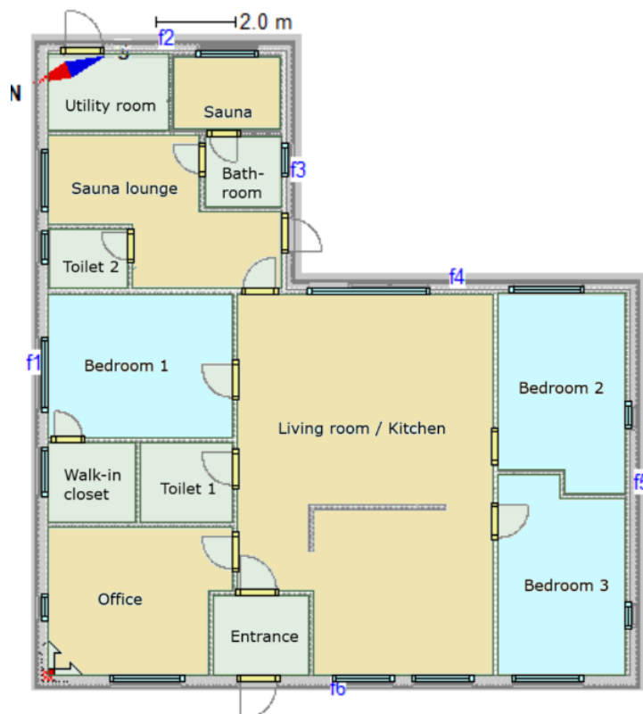
Figure 3. Zonal division of the single-family house for demand-controlled ventilation simulations.
