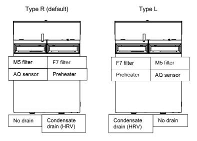
ERV (humidity recovery) model is not equipped with condensate drainage, only HRV model requires condensate removal
